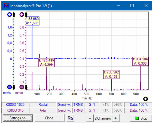
Simultaneous analysis of up to 4 signals, phase display switchable
