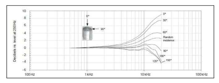
Free-field corrections for different angles of incidence
