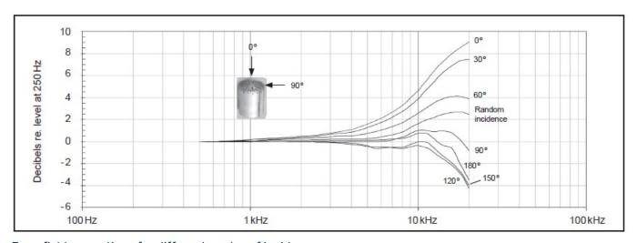
Free-field corrections for different angles of incidence
