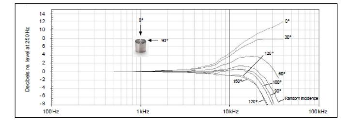
Free-field corrections for various degrees of incidence
