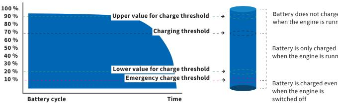
Battery does not charge when the engine is running
