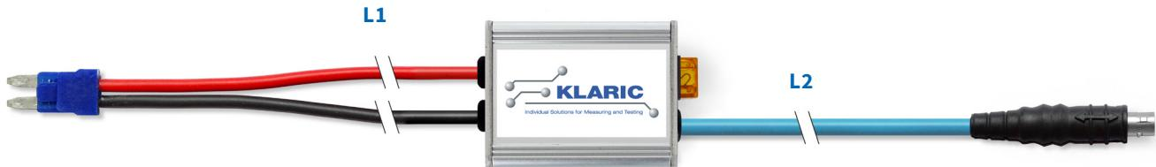
MICRO2 Fuse probe for current measurements in the fuse box with protection by the original fuse. The FK1 fuse is inserted into the fuse holder in the aluminium housing. Automatic Probe identification.
