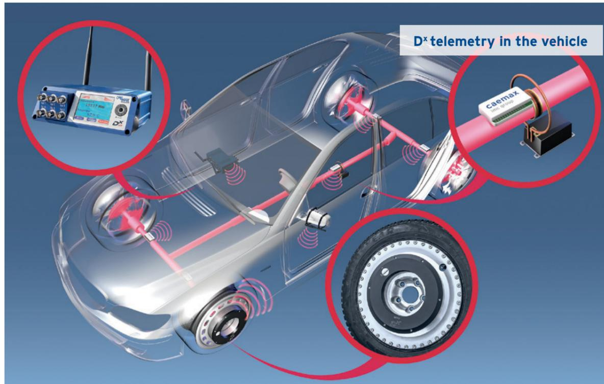
The wheel torque transducer is equipped with a modular D<sup>x</sup> telemetry digital transmitter unit. This allows for absolutely synchronous data acquisition from several transmitters in a single frequency band (868 MHz, or alternatively 2.4 GHz).
