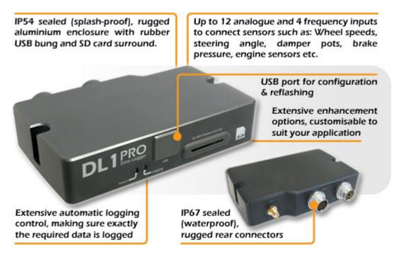
DL1 PRO the professional choice. A rugged CNC'd aluminium enclosure houses a powerful data logger, offering a huge range of enhancement options and powerful live data processing.
