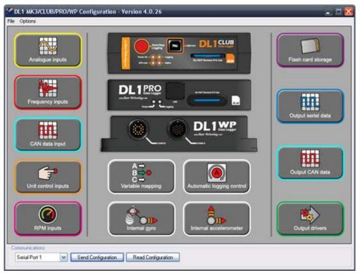
Configure the unit over USB with the user friendly configuration software
