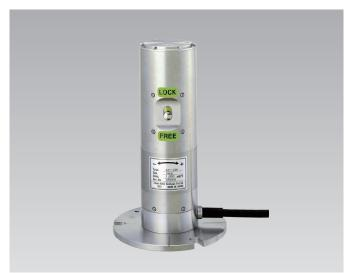
The KB-AB and KB-AC are low-capacity inclinometers. They are used to monitor the conditions of inclination of neighboring structures built by urban civil engineering works. The KB-AB measures inclination in one direction, while the KB-AC measures inclination in both X and Y directions. Protection ratings: IP67 equivalent
