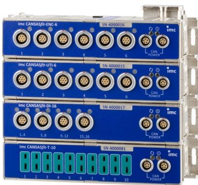
imc CANSASfit modules connected in a block
