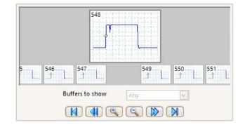
When the trace length is set to be shorter than the scope's memory, the PicoScope will automatically configure the memory as a circular buffer, recording recent waveforms for review. For example, if 1 million samples are captured, up to 500 waveforms will be stored in oscilloscope memory. Tools such as mask limit testing can then be used to scan through each waveform to identify anomalies.
