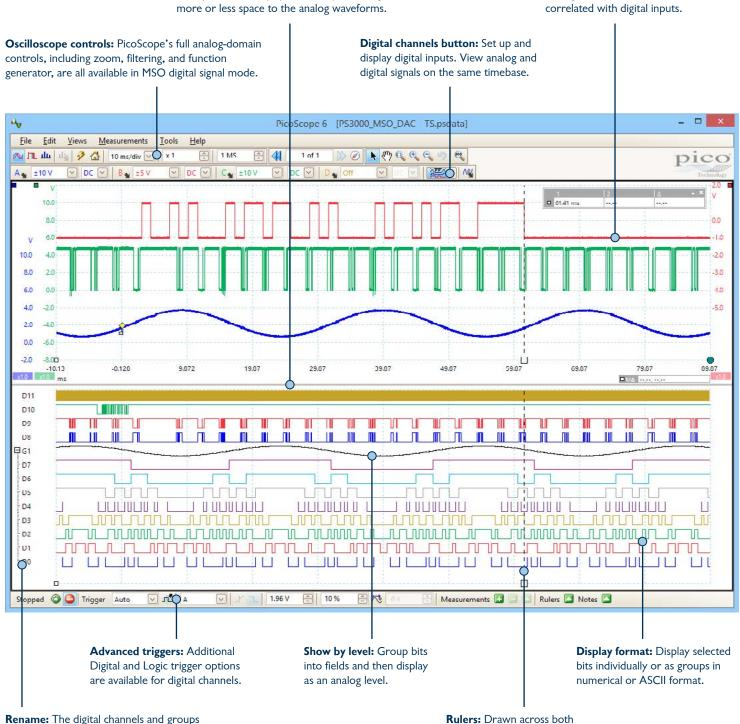
**Rename:** The digital channels and groups can be renamed. Groups can be expanded or collapsed in the digital view.
