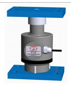
In the diagram to the left showing the CSC in a Type 3 Mounting the CSC is able to move in any direction to accommodate expansion as above. The Type 3 mount is ideal for tanks and hoppers where restraint is provided by a Type 1 or 2 mount fitted to other supports or other restraining methods are used. It is easily installed and protected with a durable 2 coat paint system meeting ISO12944/C4, medium exposure, for extended life.
