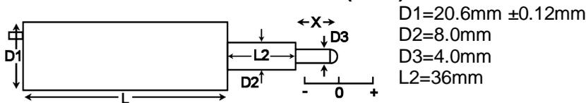
Our DCTH spring displacement transducer has bearings to guide the armature inside the measurement sensor and a spring which pushes the armature to the fully out position. Our DCTH spring return LVDTs are appropriate where it is not possible to connect the transducer armature to the moving component being measured.
