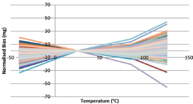
Figure 5.15 Accelerometer Y Bias vs Temperature (±10g)
