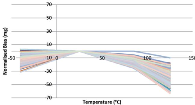
Figure 5.17 Accelerometer X Bias vs Temperature (±10g)
