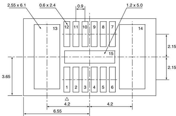
Figure 7.2 Recommended Pad Layout
