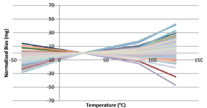
Figure 5.16 Accelerometer Y Bias vs Temperature (±2.5g)
