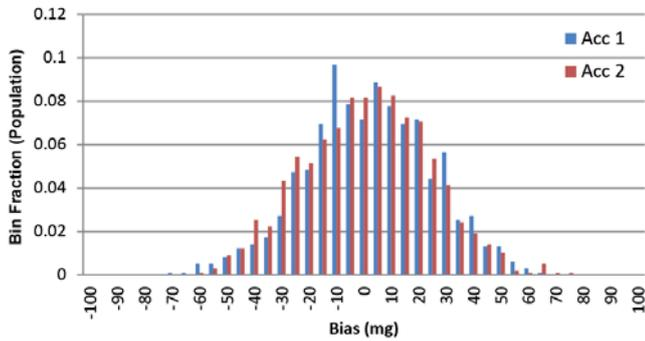
Figure 5.13 Acceleration Bias Distribution at 25°C (±10g)
