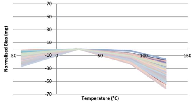
Figure 5.18 Accelerometer X Bias vs Temperature (±2.5g)
