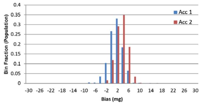
Figure 5.14 Acceleration Bias Distribution at 25°C (±2.5g)
