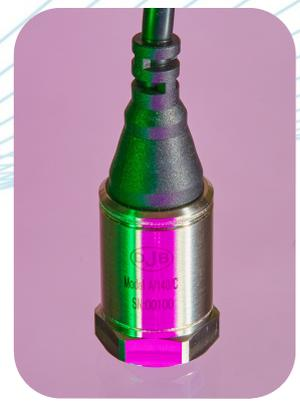
Low cost general purpose integral cable IEPE industrial accelerometer with isolated AC output. Manufactured in stainless steel for long term vibration analysis in harsh environments. Sealed to IP67 and includes 3m integral cable as standard (*additional cable can be ordered*).
