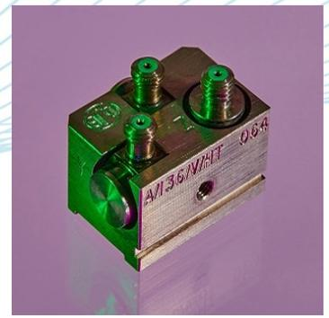
Triaxial vibration transducer comprising of three independent Konic Shear IEPE voltage output piezo-tronic accelerometers mounted orthogonally within a titanium block. Each sensor has a fully welded construction and each axis is calibrated individually in addition to the block calibration.
