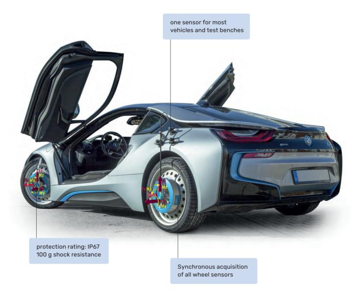
With the flexible adapter system, the WFT-C $^{\times}$  can be used with minimal effort on a variety of vehicle types - **FROM COMPACT CARS TO SUVS** and light trucks - even on the test bench. A quick system setup and convenient software functions, such as zero calibration, allow the system to be test-ready within a very short time
