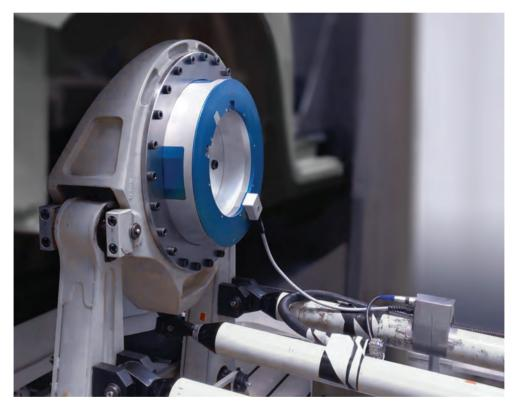
A WFT for component lifetime **TESTING ON THE TEST STAND** must be durable. Especially for these applications, imc offers WFT sensors made of titanium or steel. If a rotating measurement is carried out on a chassis dyno or on a road test, the wired signal transmission to the control unit is simply replaced by a stator. Since all of the WFT sensor housing types have the same dimensions, existing adapters can be used for all types.
