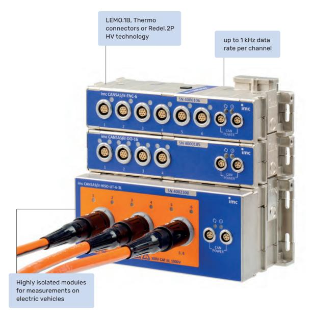
Measurement modules used for DAQ in mobile testing must be **ROBUST** and **COMPACT** because they are often placed in areas such as the engine compartment where space is limited and temperatures can be high. The imc CANSASfit series works reliably from -40° to +125° C, has a protection rating of IP65 and, due to their small form factor, can be placed almost anywhere.
