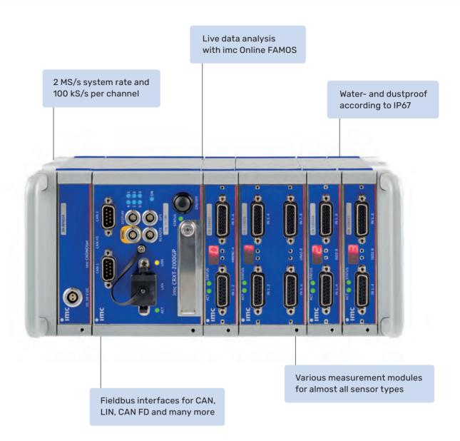
No more compromises: With the imc CRONOS-XT, imc is offering an **ULTRA-ROBUST DAQ** system in a configurable platform. Customize your data acquisition system to your needs. In addition to the base unit (data logger), you can choose from numerous universal and specialized precision measuring amplifiers. With protection class **IP67** and **MIL-STD810F**, the system is protected against dirt, dust and water as well as severe shocks and vibrations.
