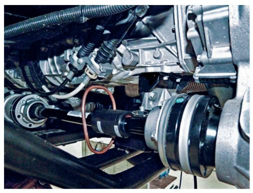
D<sup>x</sup>-Power in operation with ring stator for inductive supply
