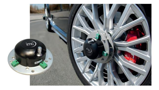
The D<sup>x</sup>-BrakeTemp is a high-precision tool for measuring temperatures on the wheels of road vehicles. All measurement signals, such as the temperatures at the brake disc, are **DIGITIZED DIRECTLY AT THE WHEELS** and transmitted telemetrically via vehicle mirror antennas to the receiver unit inside the vehicle. With its robust design, the system is also well-suited for harsh environments and road driving.
