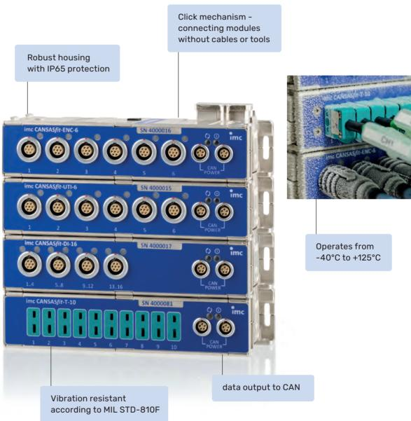
The user can simply click modules together to create blocks. Wiring between the modules is not necessary. The modules allow for direct connection to all typical sensors such as voltage, current, temperature, rpm, displacement and velocity. The digitized signals are output on CAN and can be read or recorded by any datalogger, PC or control system with a CAN interface.
