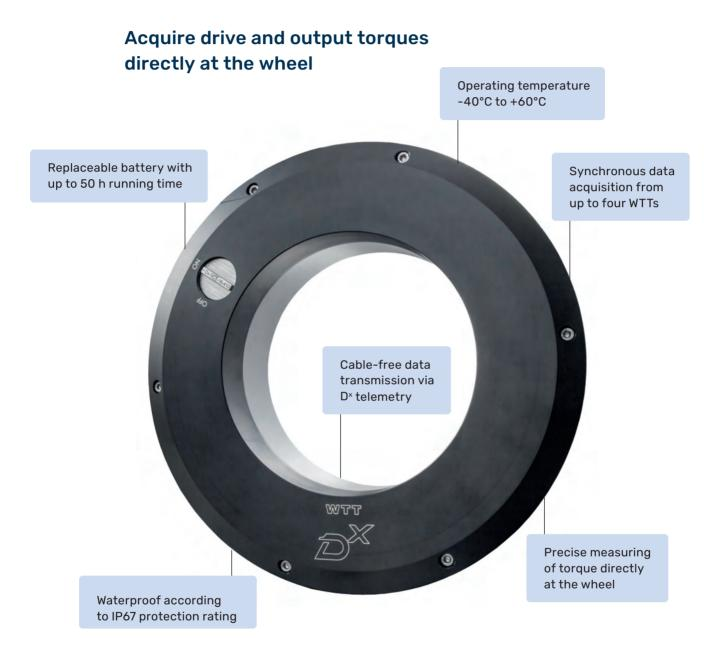
In automotive development, it is important to know the **EXACT TORQUES** acting on the vehicle – especially under acceleration and braking maneuvers. With the WTT-D<sup>x</sup> wheel torque transducer, a high-precision tool is available for making such measurements. The WTT detects the mechanical load directly where it is produced: the wheels that form the interface between the vehicle and the road.
