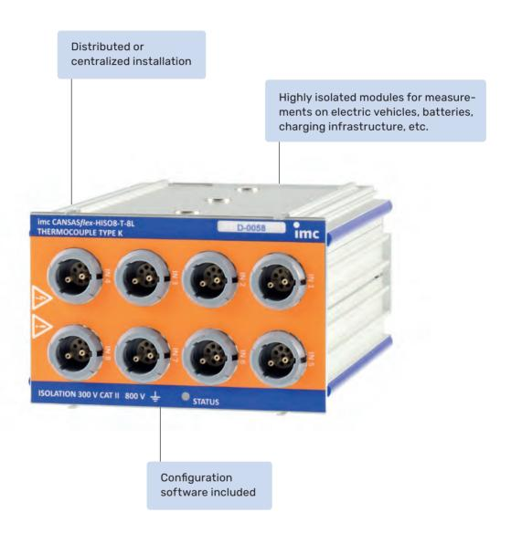
imc CANSASflex offers not only precise and versatile signal conditioning and digitization for CAN based data acquisition but can also deliver immediate results: with virtual channels, calculated directly in the measurement module up to full and comprehensive live analysis with imc Online FAMOS, provided in conjunction with imc CAN loggers such as BUSDAQflex.
