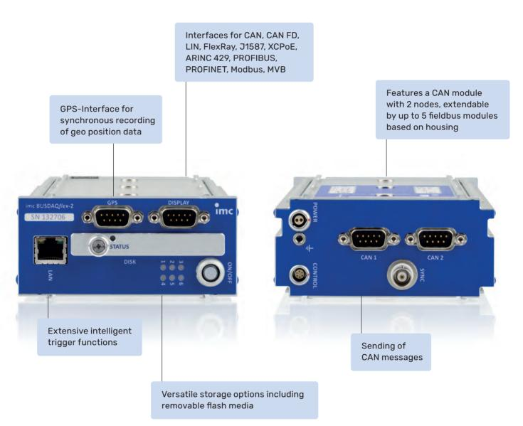
In addition to the acquisition of raw data streams and protocol channels, the **REAL-TIME DECODING** of individual channels as well as complex protocols such as CCP, KWP2000, XCP, OBD2, etc. are supported. The data logger is perfectly complemented by the imc CANSASflex measurement modules.
