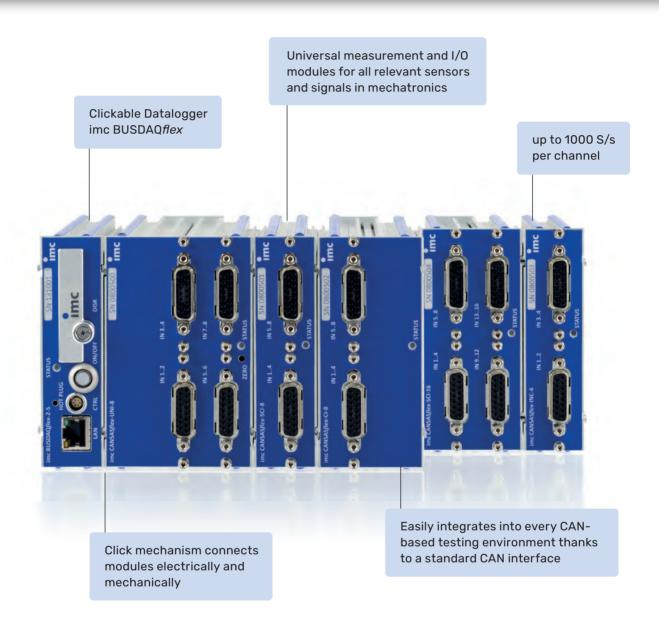
The imc CANSAS flex series offers a wide selection of can-based DAQ modules, which cover all typical sensors and signals from heavy machinery, industrial installations and vehicles. The modules can be **DISTRIBUTED SPATIALLY VIA CAN** cable or clicked together as a central unit. imc CANSAS flex modules are designed to fit into a special 19" subrack solution.
