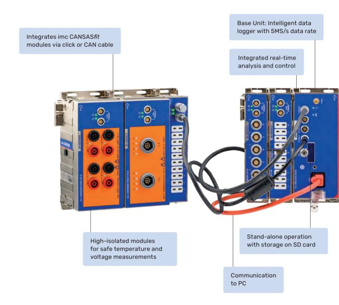
imc ARGUSfit is a **POWERFUL**, **ULTRA-COMPACT** and **FLEXIBLE** DAQ system where you easily connect the modules with a click mechanism. With high channel density, compact design, and stand-alone operation, it enables precise measurements in a wide range of applications – from prototype testing to monitoring machines and equipment.
