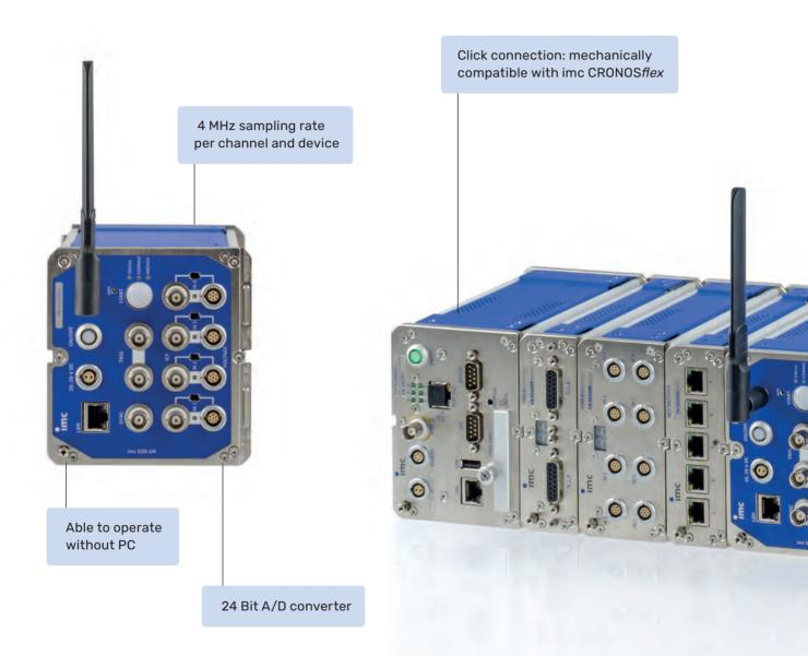
Thanks to **HIGH-SPEED DAQ** technology and versatile measurement inputs, imc EOS enables very fast and precise measurements of voltage, current transducers and IEPE sensors for acceleration, sound or force with up to 4 MHz. imc EOS is thus particularly suitable for the analysis of very dynamic processes in blast tests, material and component testing or vibration analysis.
