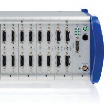
Expandable via plug-in modules or distributed synchronous CRFX modules (EtherCAT based)
