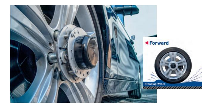
The D\*-Speed system conveniently acquires the wheel speed directly on vehicle wheels. The system does not require a stator or additional reference point and delivers measurement results – both on the test bench and outdoors – even in **HARSH CONDITIONS** such as mud, snow and dust. The accouracy ist typically better than 0.5%. Impacts against the axle also will not affect the results. This means that even driving on rough roads is possible!
