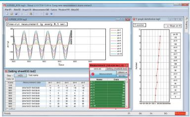
Free run measurement eliminates standby time and provides the fastest continuous measurement in the operating environment.Compatible with TS-960/-963 and TDS-630's high-speed repeatability of 0.1 second for up to 1000 points, enabling measurement at 0.1-second intervals.
