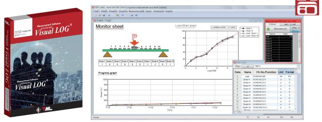
The TDS-7130v2 runs on a MS Windows PC to perform static measurement using TML data loggers. In addition to visual representation with multiple graphs, this software is a powerful tool for creating a report with data and graphs because it is capable of pasting multiple graphs, value monitors, labels and images on one graph sheet. It can take the most advantage of the data logger function of automatic multi-channel measurement.
