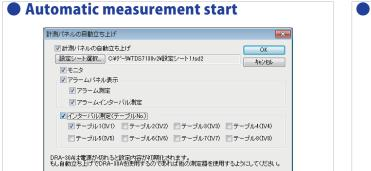
Automatically enters the measurement state when the specified setup sheet is read. Can be used for automatic recovery from power failure.
