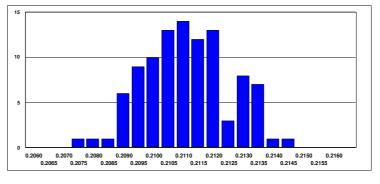
system) the integrator is adjusted to suit the coil. We also have an interchangeable coil system which can be used with appropriately-designed integrators. This allows coils to be replaced or interchanged between integrators without the need to re-calibrate the integrator. The figure shows the spread in mutual inductance values for a batch of 100 Type 1012 coils manufactured at the same time.
