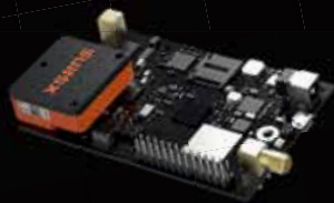
MTi 600-series Development Kit: MTi, Development board, UART2USB, USB cable (MTi-670-DK: GNSS daughter card, GNSS antenna)
