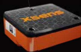
MTi enclosed: 28x31.5x13 mm, <10g, 16-pins header
