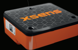
MTi encased: 28x31.5x13 mm, <10g, 16-pins header
