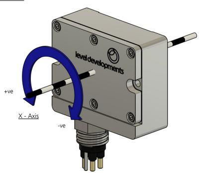
Note: only the X axis can be used when mounted vertically & the accuracy can't be guaranteed because calibration is performed horizontally.
