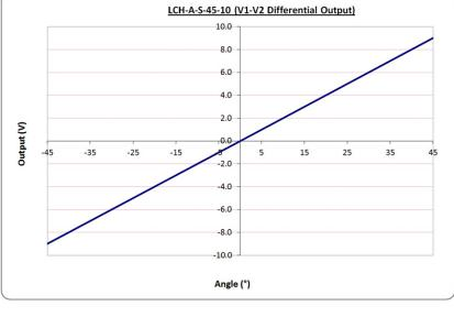
Differential Voltage output between V1 and V2 for a ±45° device with a 0.5-9.5V output interface
