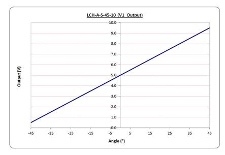
Voltage Output from V1 for a  $\pm 45^{\circ}$  device with a 0.5-9.5V output interface
