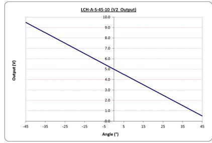
Voltage Output from V2 for a ±45° device with a 0.5-9.5V output interface
