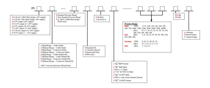
Examples: P963-0025-150PSS = 0 to 5V output from 18 to 32V supply, connector outlet, screwed in ¼" NPT port, 150 psi sealed gauge P914-0001- 2.5BAA = 20mV output, connector outlet, welded ¼" BSP female port, 2.5 bar absolute
