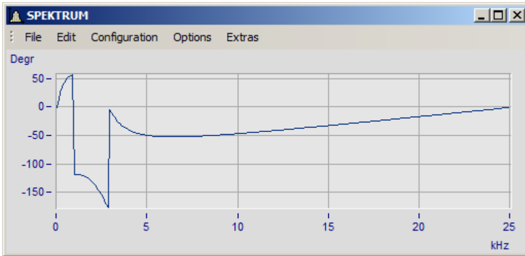
Curve window with phase of spectrum, unscaled
