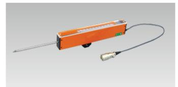
The SDP-C displacement transducer is a general-purpose, strain gauge type transducer. Designed with a strain-generating cantilever, it is able to make stable measurement while maintaining the high sensitivity to minuscule displacements.
