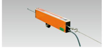
The SDP-CT displacement transducer is a general-purpose, strain gauge type transducer, and features measurement of tension displacement using hook bolt. Designed with a straingenerating cantilever, it is able to make stable measurement while maintaining the high sensitivity to minuscule displacements.
