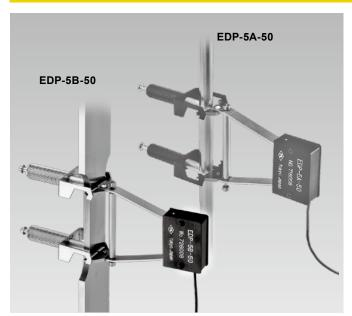
The EDP series Displacement Transducer is designed to measure elongation in round metal rod and sheet metal test specimen. It has a special holder that simply and securely holds it in place, and it detects elongation in test specimen based on displacement between two knife edges. This series uses a strain gauge for the sensing element and can be connected to an ordinary strainmeter for high precision measurements.
