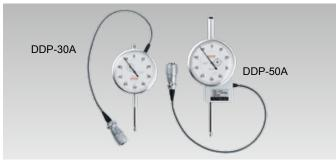
The DDP-A displacement transducer is a dial gauge with a strain sensing element and a bridge circuit integrated. The amount of displacement can be checked by viewing the pointer while the output from the sensing element can be used to control a recorder or a machine. Protection ratings: IP40 equivalent
