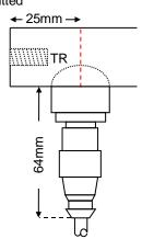
Cable length 5m Operating temperature range\* -25°C to 90°C Maximum static pressure\* 1000kPa M5x0.8, 11mm
