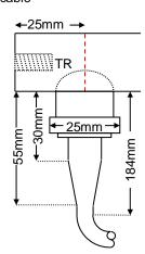
Cable length 600mm to 7m Operating temperature range\* -40°C to 100°C Maximum static pressure\* 3MPa M5x0.8, 11mm
