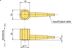
The ARE-A acceleration transducer is used to measure the acceleration of structures subject to relatively strong vibration. It is small, lightweight and easy to operate.
