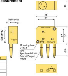
Input/Output cable : ø 3.2mm 0.08mm<sup>2</sup> 4-core shielded vinyl cable 5m Input/Output cable is grounded to the body.
