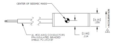
Direction of measurement must be specified at time of order.
