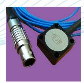
The AMT range of accelerometers are Triaxial MEMS (micro electro mechanical system) DC response voltage output devices for testing at low frequency vibration measurement from DC (0Hz) and above. They are Triaxial (measuring in 3 directions simultaneously) variable capacitance design and are available with a 2m integral cable fitted with a 7pin connector to suit the DJB DCM-03 MEMS signal conditioning unit or alternatively as bare wires.
