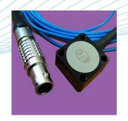
The AMB range of accelerometers are Biaxial MEMS (micro electro mechanical system) DC response voltage output devices for testing at low frequency vibration measurement from DC (0Hz) and above. They are Biaxial (measuring in 2 directions simultaneously) variable capacitance design and are available with a 2m integral cable fitted with a 7pin connector to suit the DJB DCM-03 MEMS signal conditioning unit or alternatively as bare wires.
