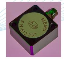
The AMB range of accelerometers are Biaxial MEMS (micro electro mechanical system) DC response voltage output devices for testing at low frequency vibration measurement from DC (0Hz) and above. They are Biaxial (measuring in 2 directions simultaneously) variable capacitance design. The AMB/50.40C has a 4 pin ½-28UNF side entry connector.
