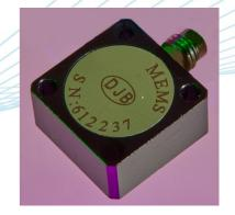
The AMB range of accelerometers are Biaxial MEMS (micro electro mechanical system) DC response voltage output devices for testing at low frequency vibration measurement from DC (0Hz) and above. They are Biaxial (measuring in 2 directions simultaneously) variable capacitance design. The AMB/30HR.66C has a 4 pin ½-28UNF side entry connector.
