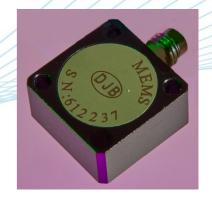
The AMB range of accelerometers are Biaxial MEMS (micro electro mechanical system) DC response voltage output devices for testing at low frequency vibration measurement from DC (0Hz) and above. They are Biaxial (measuring in 2 directions simultaneously) variable capacitance design. The AMB/200HR.10C has a 4 pin ½-28UNF side entry connector.
