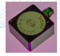
The AMB range of accelerometers are Biaxial MEMS (micro electro mechanical system) DC response voltage output devices for testing at low frequency vibration measurement from DC (0Hz) and above. They are Biaxial (measuring in 2 directions simultaneously) variable capacitance design. The AMB/200.10C has a 4 pin ½-28UNF side entry connector.
