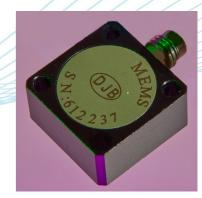
The AMB range of accelerometers are Biaxial MEMS (micro electro mechanical system) DC response voltage output devices for testing at low frequency vibration measurement from DC (0Hz) and above. They are Biaxial (measuring in 2 directions simultaneously) variable capacitance design. The AMB/10HR.200C has a 4 pin <sup>1</sup>/<sub>4</sub>-28UNF side entry connector.
