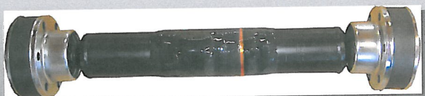
Shaft after application and calibration with waterproof and shock resistant encapsulation
