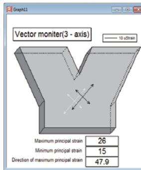
Principal stress and strain are indicated by arrow. The line color changes when the alarm condition is satisfied.
