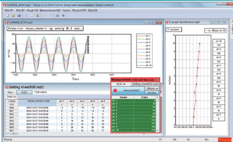
The data logger TDS-630 can make repeated measurement of up to 1000 channels by every 0.1 seconds.
