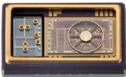
Figure 11.2 Combi-Sensor (Lid Removed)
