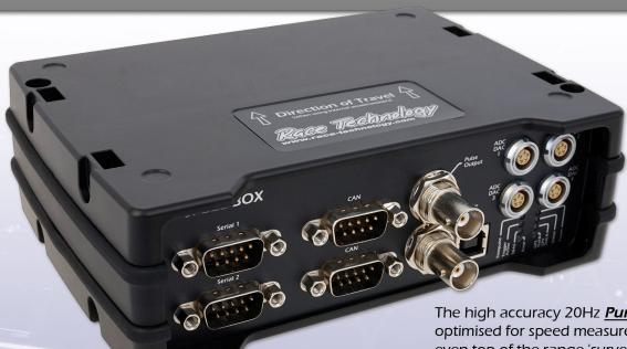
The **SPEEDBOX** and **SPEEDBOX MINI** are very high accuracy non-contact speed sensors which have been designed for professional automotive testing as well as other industrial and high-end motorsport applications. They output a low latency, non-interpolated speed measurement comprised of GPS and inertial data combined using an adaptive filter for exceptional performance even in environments where accuracy of GPS-only sensors is severely degraded.
