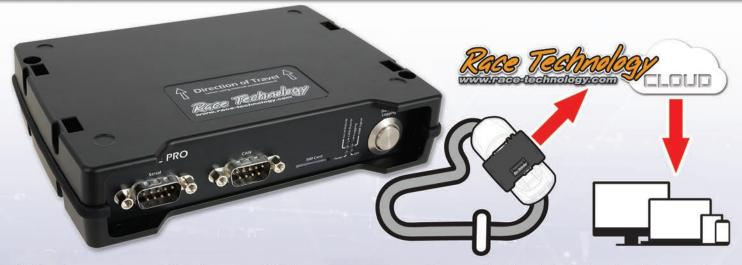
RT Live is a new type of data logger, which logs directly to a secure cloud storage using a wireless mobile internet connection. Data logged by the unit can be accessed over the internet, and all inputs to the device can also be monitored in real time over the internet using any web browser (including Microsoft, Apple and Android products), or using our PC software
