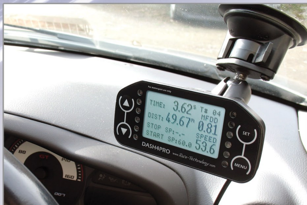
Secure temporary mounting with suction mounting kit
