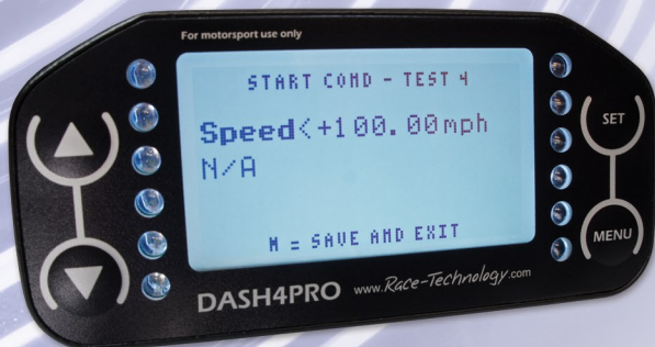
Configuring SPEEDBOX triggered tests using the DASH4PRO display
