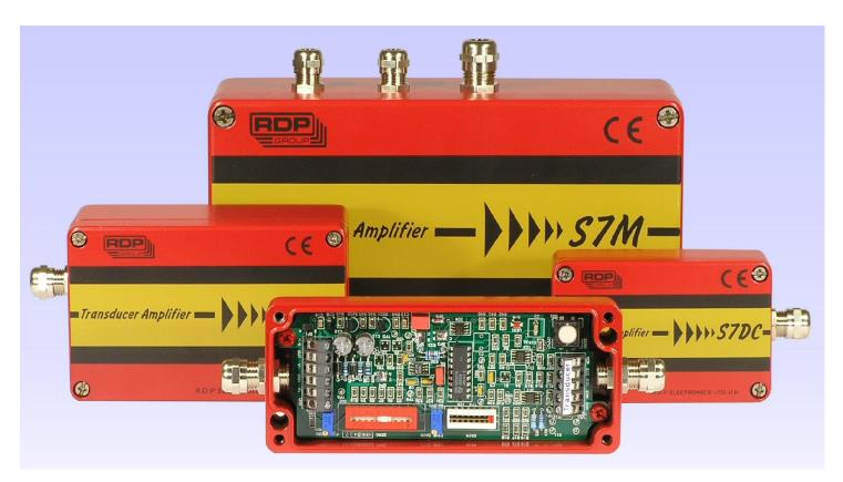
Signal conditioning is required where the output of a transducer needs to be boosted or changed into a form suitable for the monitor or logging device which will be used. These amplifiers are suitable for LVDT transducers, strain gauge sensors and some internally amplified transducers.
