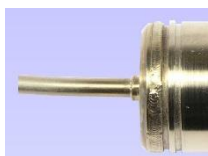
Option code 5 - End exit integral MI (mineral insulated) stainless steel cable
