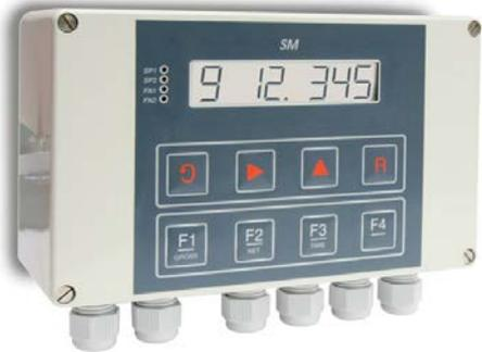
*An extremely flexible digital indicator and display system for use with a wide range of sensors and transducers including volts, amps, temperature, frequency, speed, load, force, pressure, torque, LVDT, RVDT and many more*
